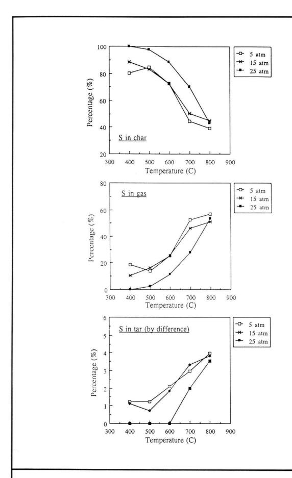
Figure 10 . Sulphur Distribution in Pyrolysis Products
