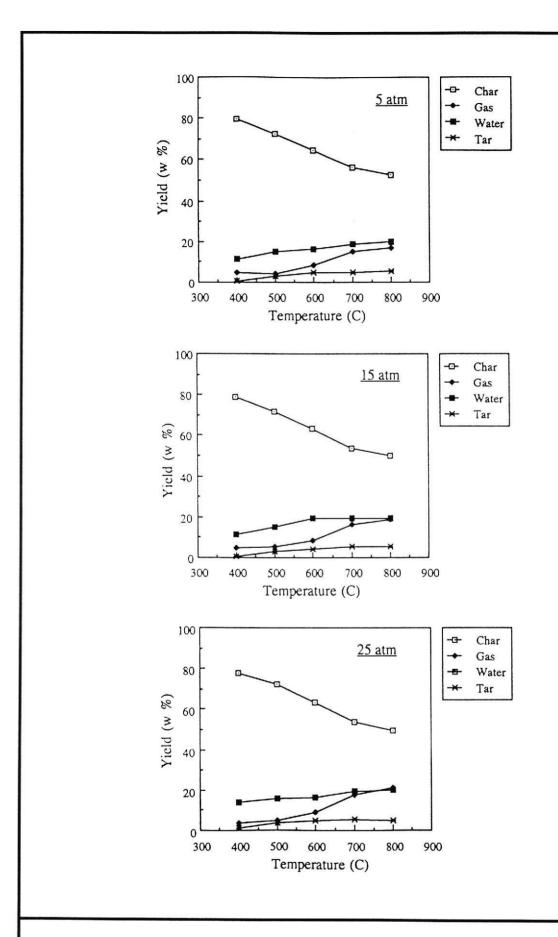
Figure 7 . Effect of Temperature on Pyrolysis Product Distribution
