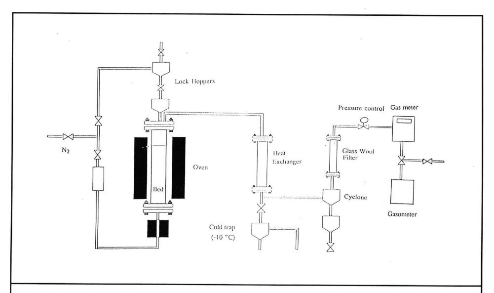
Figure 6 . Layout of the Fixed Bed Reactor used during the Pyrolysis Tests
