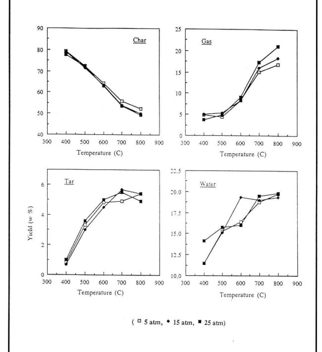
Figure 8 . Effect of Pressure on Pyrolysis Product Distribution
