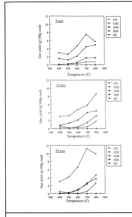
Figure 9 . Composition of Pyrolysis Gas
