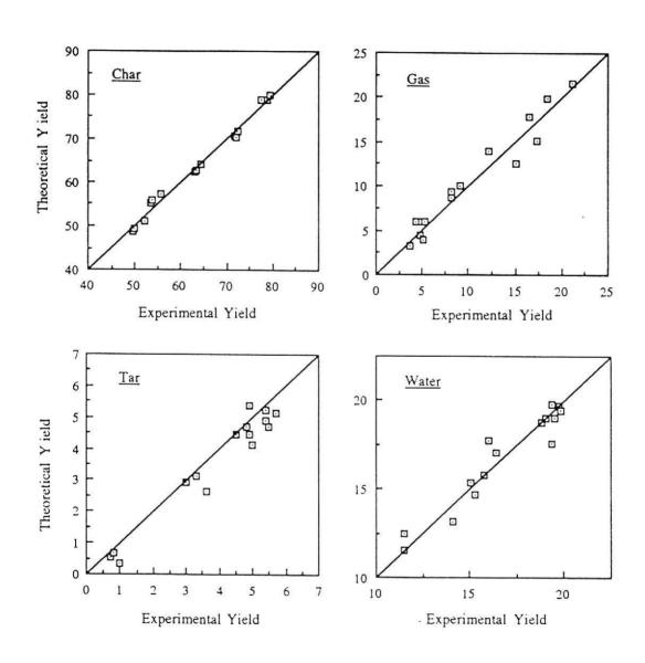
Figure 11 . Comparison between Experimental Pyrolysis Product Data and Empirical Correlations
