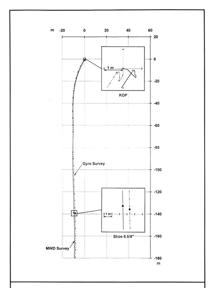
Figure 1a . Comparison of ET4 MWD and Gyro Surveys (Horizontal Section)
