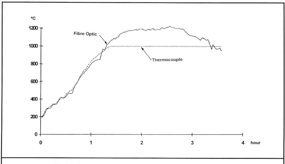
Figure 3 . Comparison between Thermocouple and Fibre Optic Measurements (temperatures versus time - temperature controlled oven)
