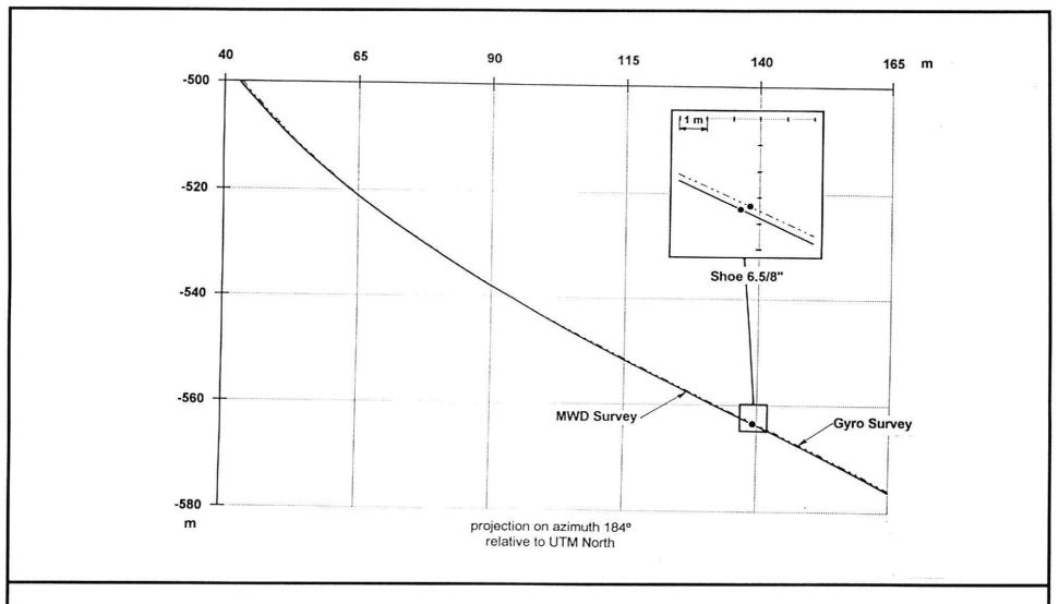
Figure 1b . Comparison of ET4 MWD and Gyro Surveys (Vertical Section - In-seam Interval)
