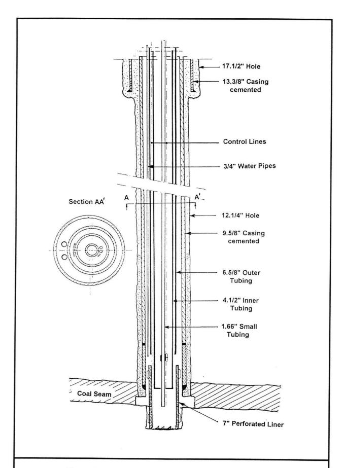
Figure 5 . Proposed Double-annulus Configuration for Recovery Well[RW(ET5)]
